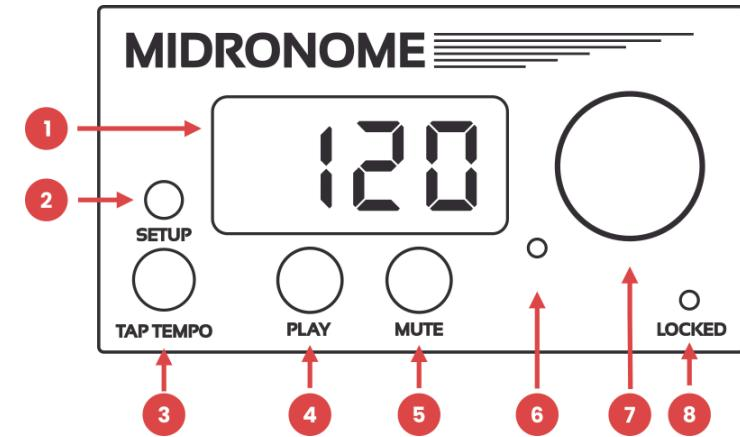
2. Setup Button - enter and leave the settings, hold down to turn off the device
